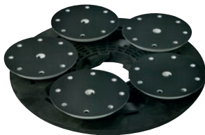
Parquet satellite disc 5E For a perfect sanding and end result of among others herringbone patterns, mosaic parquet and other pattern floors. Five counter rotating discs with double bearing on a driving disc with dust holes.
