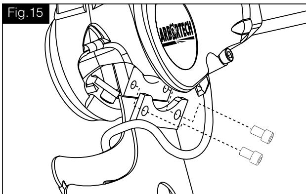
**CAUTION:** DO NOT operate the tool with loose blades. If blades should come loose while operating, the blade mounts and threads can become damaged, requiring significant repairs to the tool.
