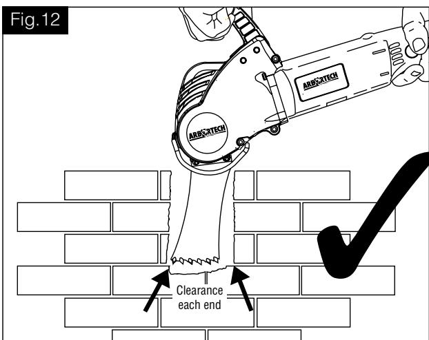
When using the Mortar Plunge blades, the cut should have enough clearance on each end (shown in fig:12), to ensure that no hammering of the blade ends occurs (as shown in fig.13).
